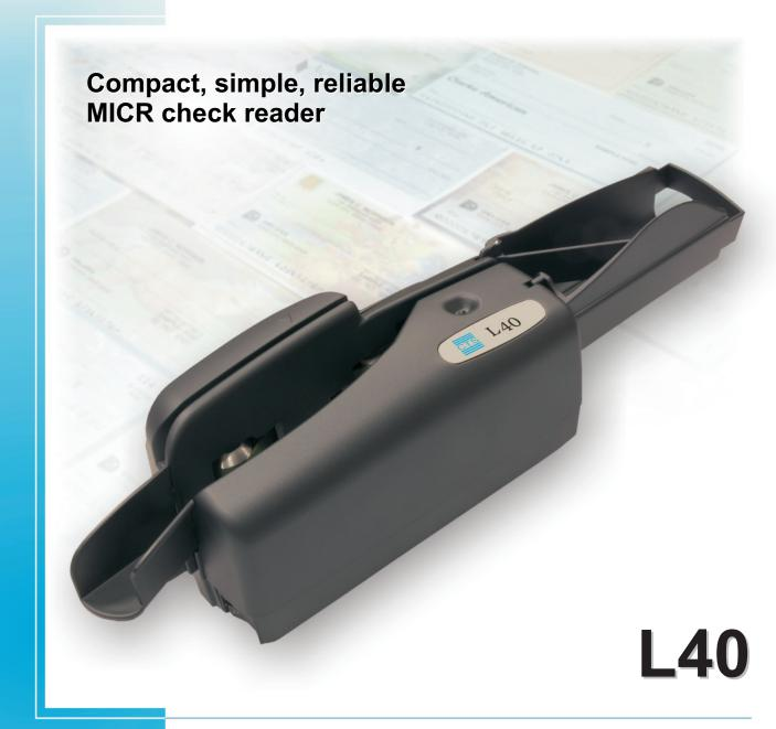
The L40 document reader is an innovative entry level MICR check reader designed for an easy connection to the host - plug & read -, an automatic drop and feed mechanism (pinch roller) and a friendly layout.
